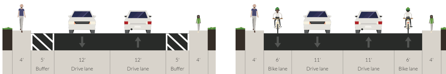
Cross section of Route 135 showing existing condition with no left turn lane (left) and Option 1 with two one-way in-road bike lanes.
