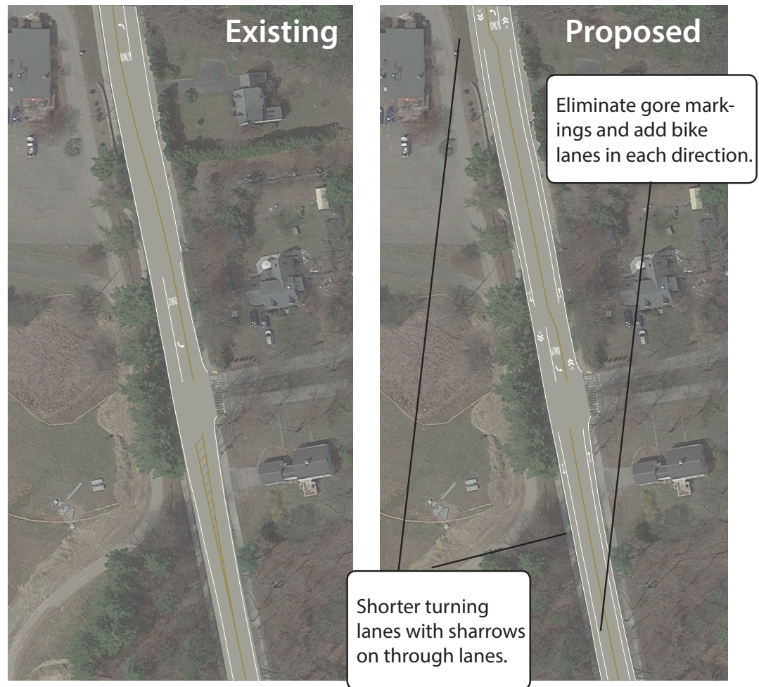
Existing and proposed Speen Street roadway configuration, illustrating addition of bike lanes.
